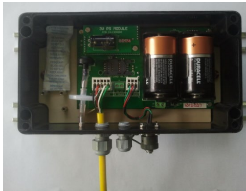
Figure 5-1 Datalogger powered with 2 x 1.5 V Alkaline Batteries
