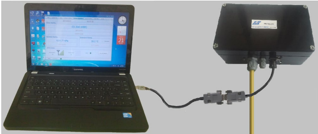
Figure 6-3: Datalogger connection using communication cable
