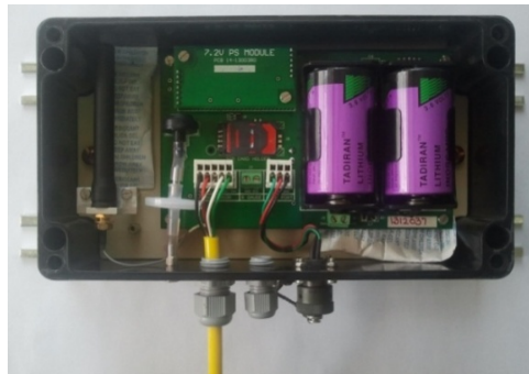
Figure 5-2 Datalogger powered with 2 x 3.6 V Lithium Batteries
